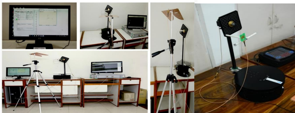
Antenna Testing and Radiation pattern measurement setup
