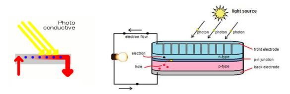
Fig. 3 Schematic and working of Photo conductive cell.
