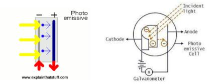
Fig. 1. Schematic and working of photo emissive cell
