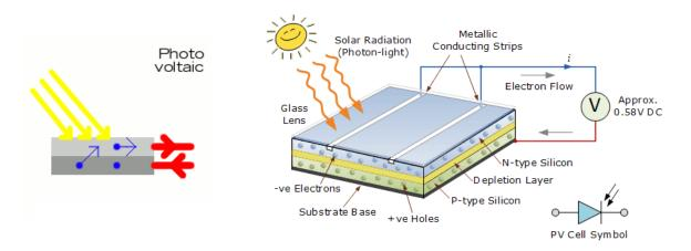
Fig. 2 Schematic and working of photovoltaic cell (Solar cell)
